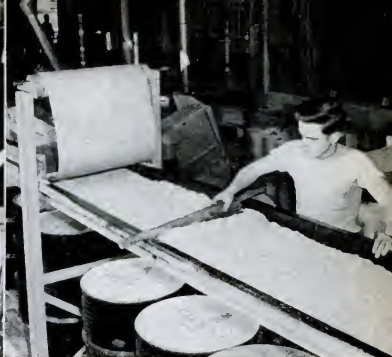
Paper makes a tray to carry the mix into the press. "Comb" in man's hand spreads it on paper while previous boards are cooking in press. This press makes two boards in each cycle.
